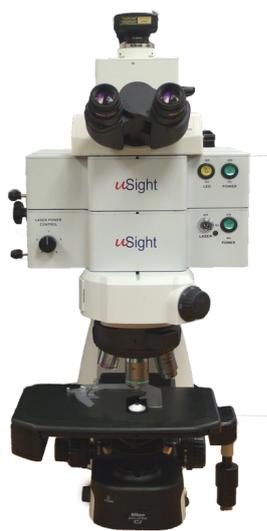
**Figure 1.** uSight-2000 and uSight-X module mounted onto a Nikon Ci-S microscope
